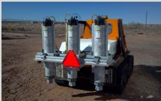
Overland Radiation Measurement System, “Orion ScanPlot SM ”
