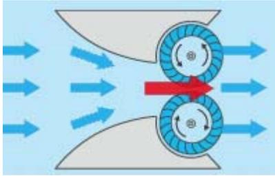
The micro-hydro system, *Stream*, is a simple system that can be installed in almost any waterway. It doesn't need a dam-based reservoir or an aqueduct. Therefore it requires no additional civil construction work, meaning a massive saving in both cost and time compared to traditional (dam based, etc.) hydroelectric systems.
